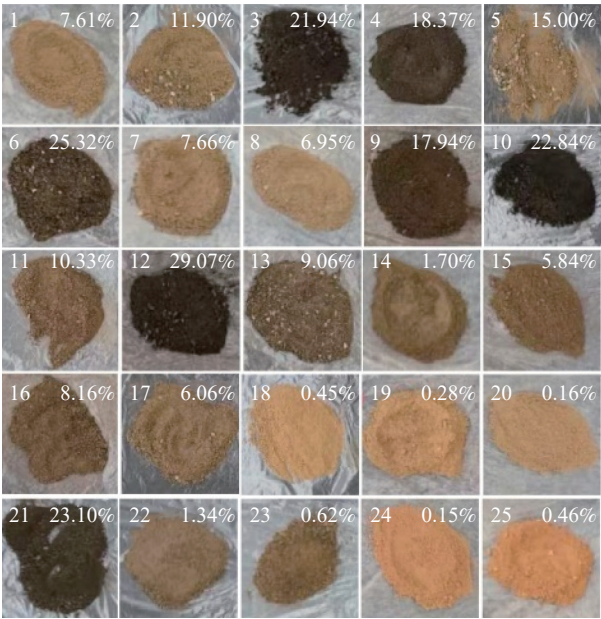
图 3 加热后的土壤样品(图中数字为土样有机质含量) Fig. 3 Soil samples after heating (numbers in the image represent organic matter content of soil samples)
