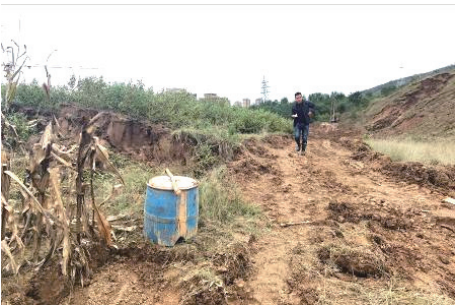
图 8 1#、2#滑块部位平台反翘 Fig. 8 Reverse warping of the platform at the locations of sliders 1# and 2#
