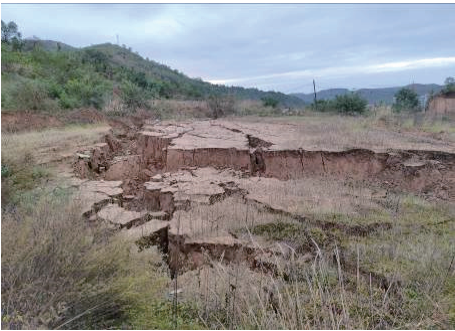
图 7 1#、2#滑块之间裂缝及地面拱起 Fig. 7 Cracks and ground arch between sliders 1# and 2#
