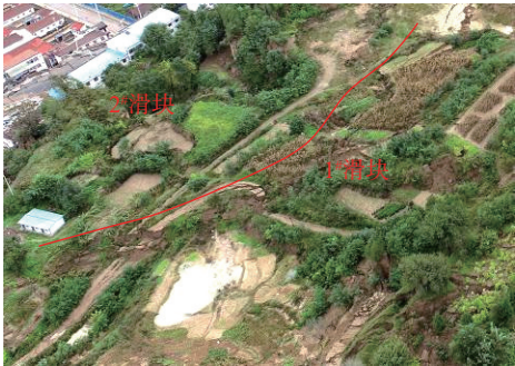
图 6 1#、2#滑块之间裂缝及相对错动 Fig. 6 Cracks and relative mismovements between sliders 1# and 2#
