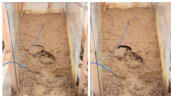
图 3 斜坡浅层局部块体滑塌形态 Fig. 3 Local block collapse form in shallow layer of slope
