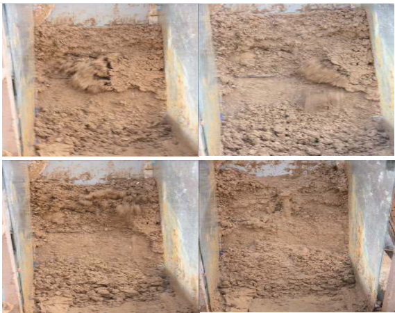
图 4 斜坡块体滑塌破坏后的形态 Fig. 4 The shape of slope block after collapse failure
