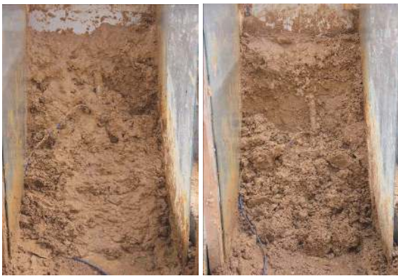
图 5 斜坡深层整体滑塌失稳破坏形态 Fig. 5 Failure pattern of overall collapse and instability of deep slope
